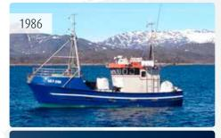
Master: Frederik Mathiassen Length/width: 14.85 x 5.16 Production capacity: None Catch capacity: 150 ton/yearly Hold capacity: 10 ton Crew: 4 men Trawler type: Coastal line/net vessel, crab vessel
