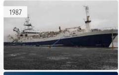
Master: Jónfrídur Poulsen Birgir Petersen Length/width: 77,6 x 12,6 m Production capacity: 120 ton/day Catch capacity: 20-25.000 ton/yearly Hold capacity: 700 tons
