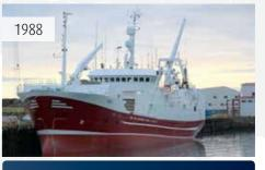
Master: Páll Johan Poulsen Length/width: 70 x 12,5 m Production capacity: 60 ton/day Catch capacity: 10-15.000 ton/yearly Hold capacity:500 tons Crew: 10-12 men Trawler type: Pelagic trawl Ownership: RG 66%
